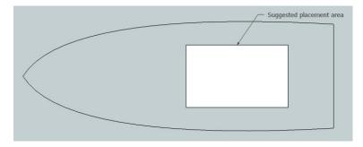
Placement – The location is not prescribed but it is suggested to mount in the central area away from other electronics. Do not mount beneath carbon fibre or any other material that will absorb the transponder signal.
